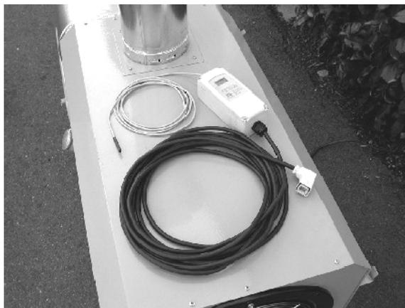
The remote thermostat sensor cable, control box, cable, and jack
