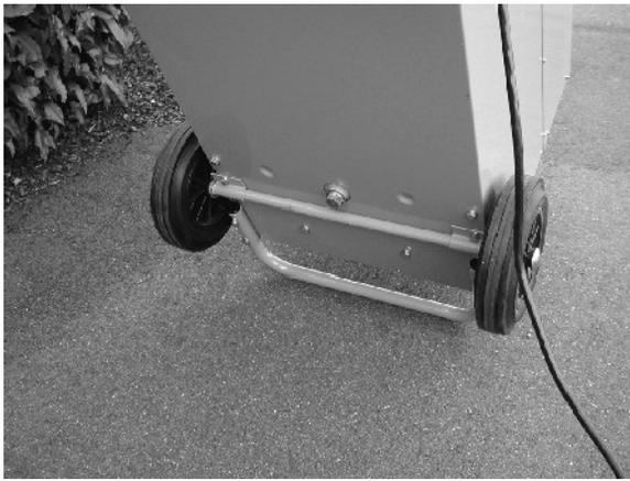
The internal fuel tank drain plug
