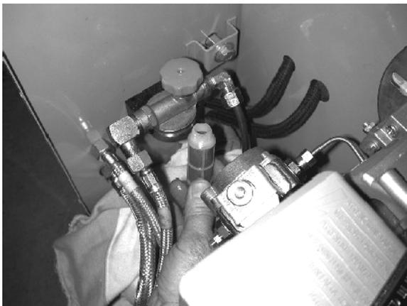
Unscrew the fuel intake filter by hand
