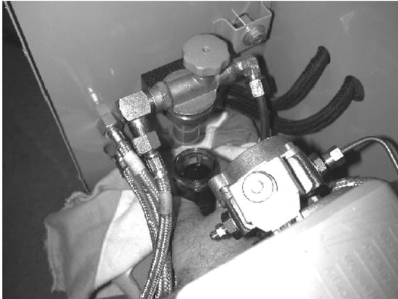
Unscrew the filter reservoir by hand
