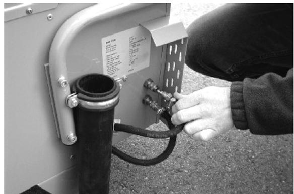
Connect the internal tank fuel lines
